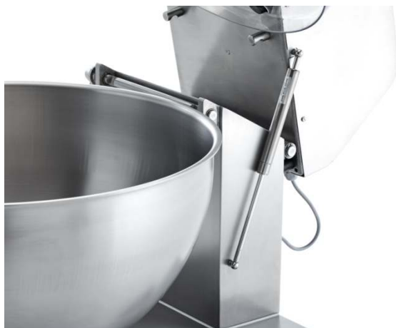
Pneumatic spring to assist raising the machine head.
